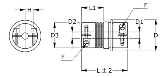
D = 94 Nom. torque NM (Tkn) = 130NM overload torque range 1
